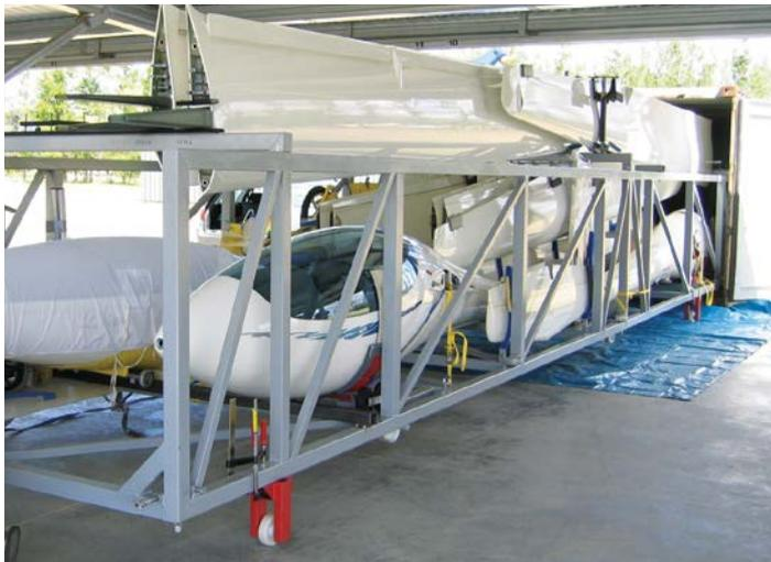
Cradle withdrawal – temporary wheels (painted red) are fitted to transfer the weight of the cradle to the floor.
